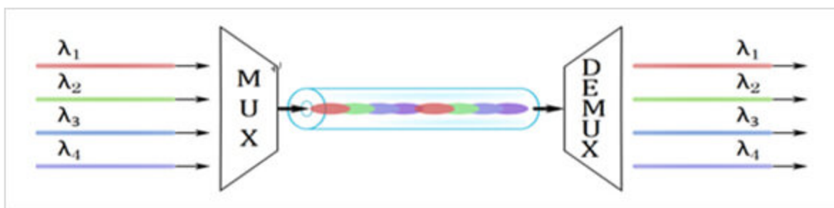
Figure 1 Shortwave Wavelength Division Multiplexing (SWDM)
