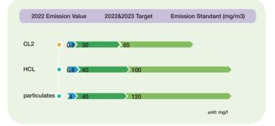
The Group continued to strengthen control measures during the operation period to ensure the compliance emission of exhaust gas. In 2023, the Wuhan headquarters of YOFC set an emission target stricter than the local emission standard.
